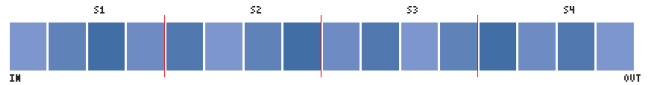
Fig. 1. A pipeline-parallel transformer with K = 4 stages. The slowest stage dominates the per-microbatch step time.
